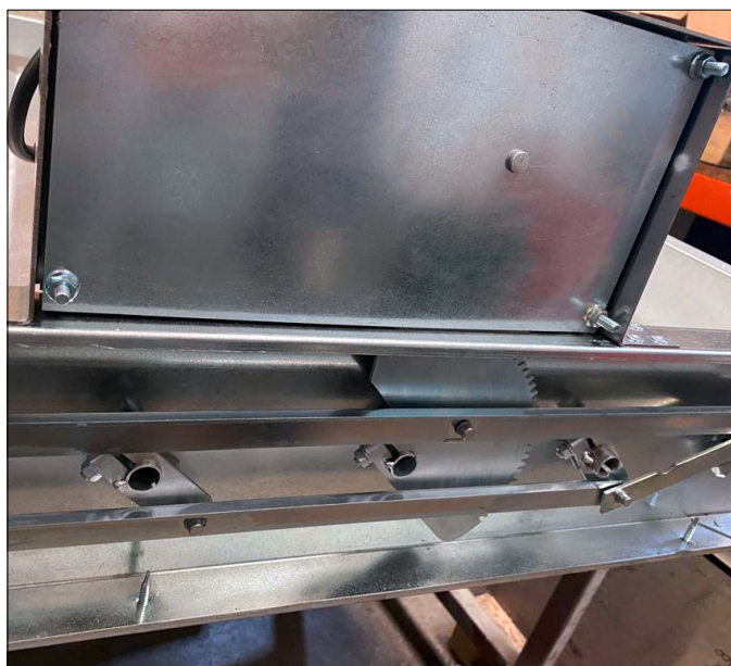
Reinforced drive shaft and Oilite bearings
