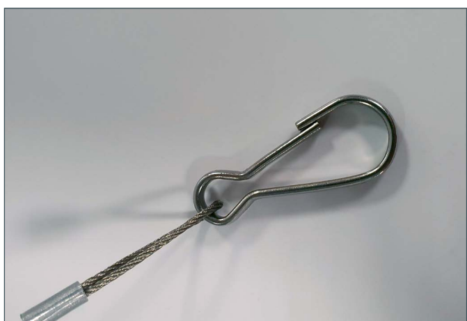
Fig. 15 Close-up of retaining wire
